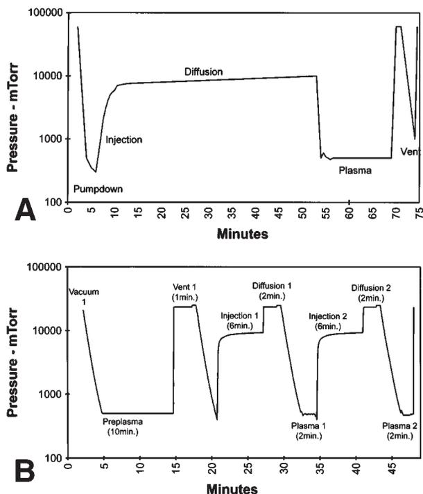
**Fig 1.** Characteristic cycle curves for the Sterrad 100 (A) and Sterrad 100S (B).
