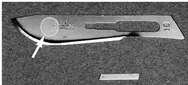
**Fig 2.** Number 10 Bard-Parker stainless steel surgical blade after being inoculated with a 10  $\mu$ l suspension of spores (arrow). This carrier was placed into the center of the LTUs (see Fig 3). In addition, a smaller stainless steel carrier cut from a number 10 Bard-Parker surgical blade is shown. This carrier was placed into the center of the straight LTUs (see Fig 3, A).
