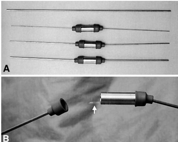
**Fig 3.** **A**, LTUs of varying diameters (diameters 1 mm, 2 mm, 3 mm), including straight LTU made of stainless steel (diameter 3 mm, top). **B**, Test objects were placed into the LTUs by aseptically unsealing the hard rubber septums connecting the stainless steel tubing.
